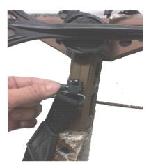
Tighten thumb screws securely on both swivels.
